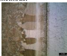
Figure 1 – Brazed seam EK-181//Cu-28Ti//V
