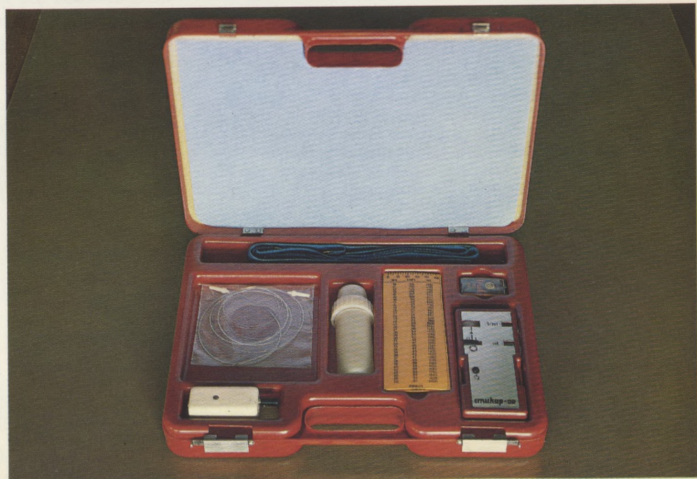
A set of equipment for checking implanted electric cardiostimulators, developed at the MEPhI
